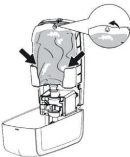
ATTACH THE POUCH WITH THE LABEL FACING THE BACK WALL TO THE HOOK AND VERIFY THAT IT FITS PROPERLY.
