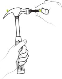
TAP ANCHORS INTO EACH DRILLED HOLE.
