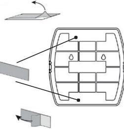
PLACE THE ADHESIVE FILM ON THE INTENDED SURFACES ON THE WALL BRACKET AND REMOVE THE PROTECTIVE FILM.
