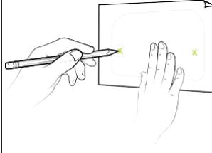
MARK THE POSITION TO DRILL WALL MOUNTING HOLES.
