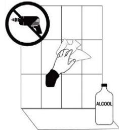
CLEAN THE SURFACE WITH A SUITABLE CLEANER. FINALLY, DRY THE SURFACE THOROUGHLY.
